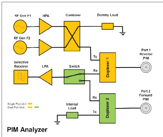
Figure 2. Block diagram of single port and dual port PIM analyzers.
