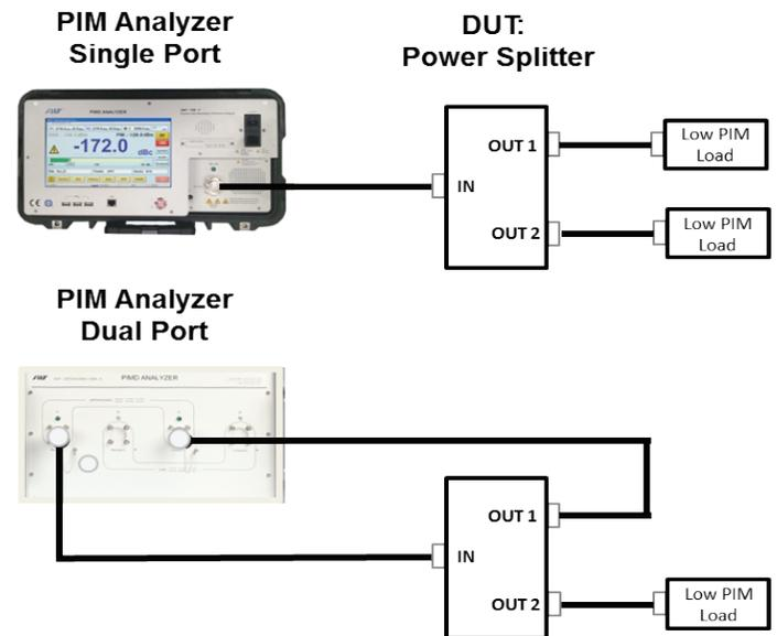
Figure 5. Forward and reverse pim measurement of a 3 port DUT (power splitter)
