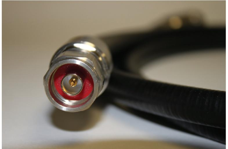
PIM is an unwanted signal distortion caused by non-linear behavior of passive components in the RF path of telecommunication systems. PIM happens when these systems carry two or more RF signals simultaneously. Multi carrier systems are the norm with today's in-building DAS installations. Not only can PIM degrade signal quality, it can affect system performance so severely that it may even drop calls. Users become disgruntled about poor service, network operators lose revenue.
