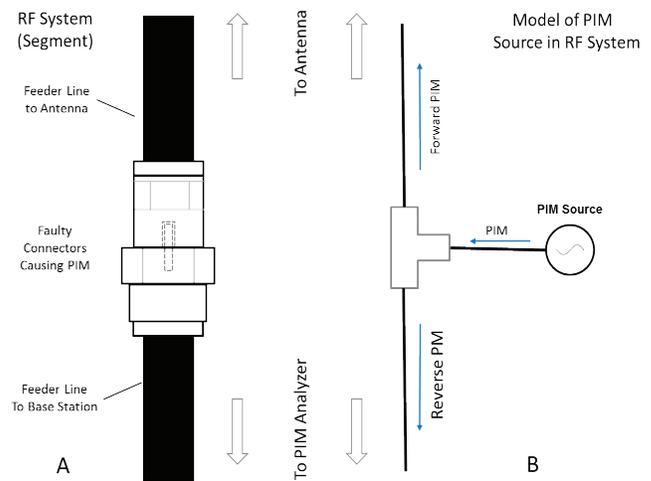
Figure 1. Electrical model of PIM source in RF system.
